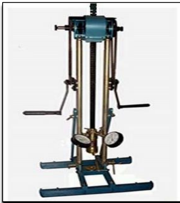
Gambar 2.1 Alat Sondir ( Cone Penetration Test ) (Sumber : http://www.ghaninusantara.com )
