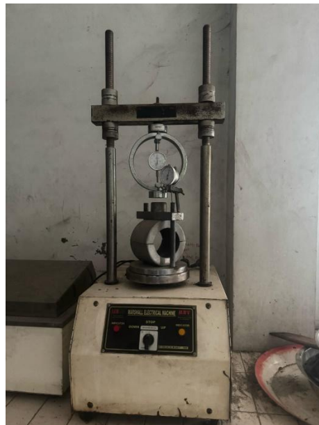
Alat Marshall Test
