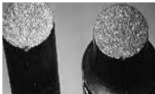
Gambar 2.21 Patah Getas ( Brittle Fracture )(Rangga Agung, 2017)
