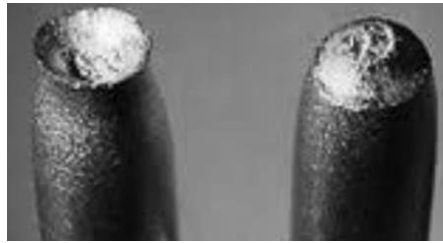
Gambar 2.23 Patah Ulet ( Ductile Fracture )(Rangga Agung, 2017)
