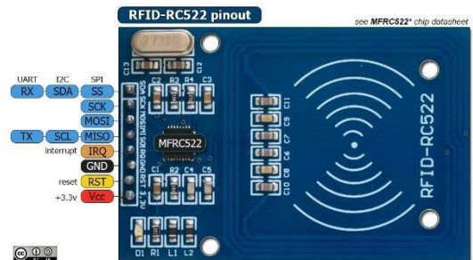
Gambar 2.1 Pin RFID Reader
