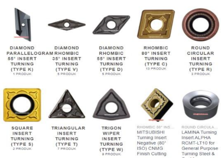
Gambar 2. 5 Mata Pahat Insert Karbida
