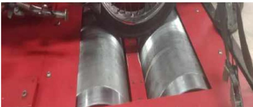
Gambar 3.2. Chassis Dynometer Sepeda Motor
