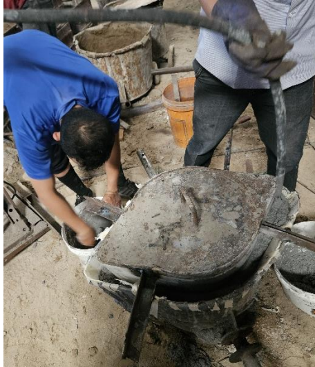
Gambar 2.7 Instalasi Lining Ladle
