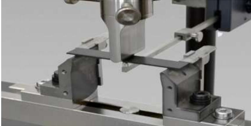
**Gambar 2.22** pengujian Bending
