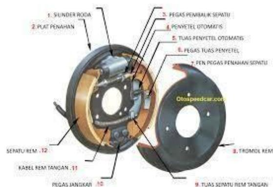
Gambar2.II.2 Keterpasangan rem tromol
