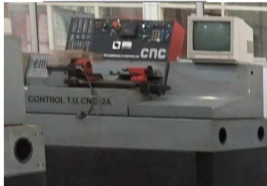
Gambar 2.5 Mesin Bubut CNC TU-2A
