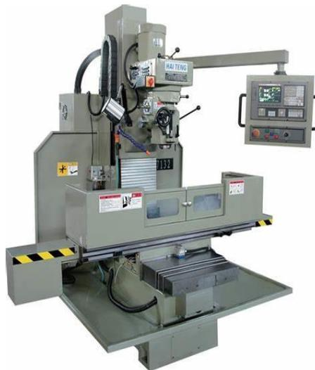
Gambar 2. 9 Mesin Frais CNC Tipe Bed (*Bed Type CNC Milling Machine*)
