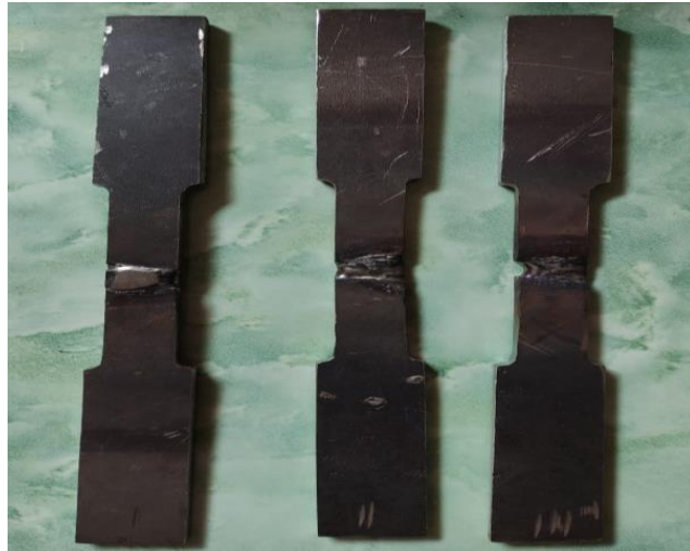
Gambar 2.5 Spesimen Uji Tarik (ASTM E8/E8M – 13a)
