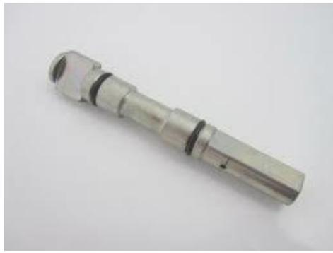
Gambar 2.6 *Brake Cam*
