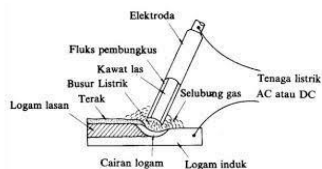
Gambar 2.1 Las SMAW (Shielded Metal Arc Welding)
