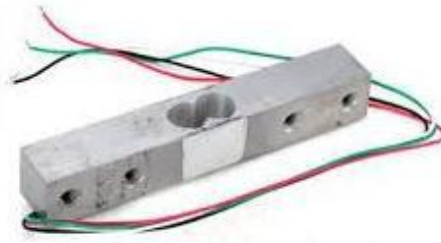
Gambar 2.4. Sensor Berat Load Cell (Nuryanto, 2015)
