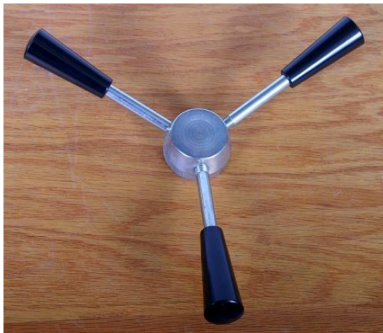
Gambar 2.6 Drill feed handle mesin bor duduk.
